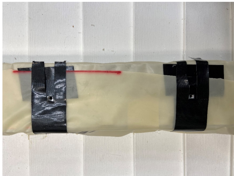
Figure 36. Reinforcement of latex with tape around fastener areas.
