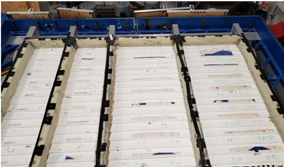
Figure 52. Exploration of failures in vinyl siding panels after ASTM 5206 testing of specimen 4.
