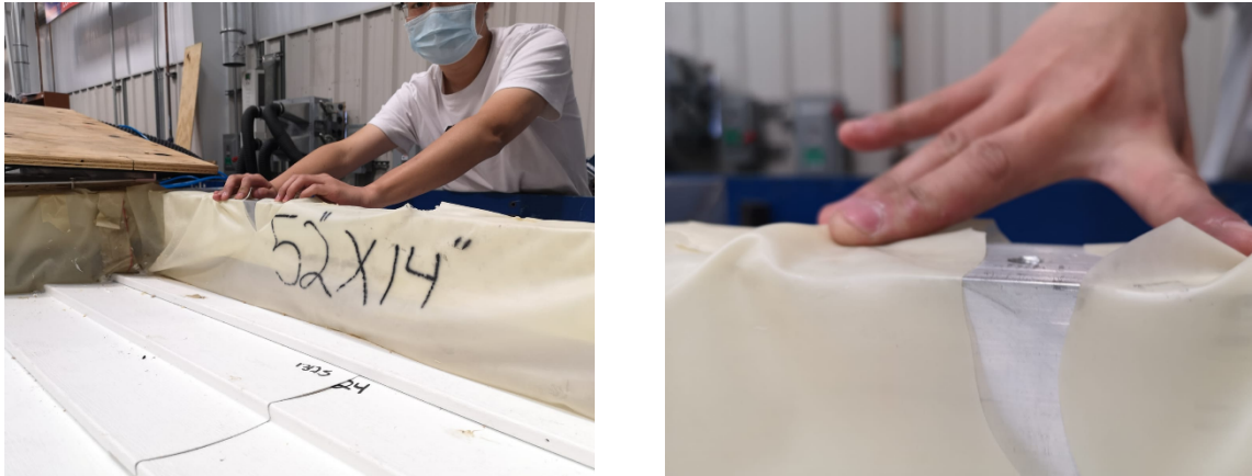
Figure 35. Failure of latex in fourth chamber specimen 1 on July 8, 2020; possibly due to fastener penetration through the latex.
