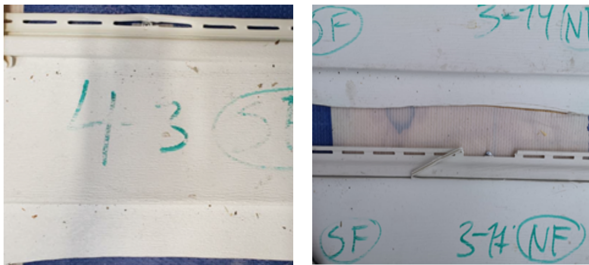
Figure 34. Typical failure modes encountered during ASTM D5206 testing. Vinyl siding panels stretch as pressure is applied and slide through the fastener (SF) (left image); rupture of the nail hem (NF) (right image).
